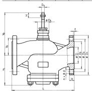
with regard of the standard previously in force, there is an option to have the number of connection bolts as stipulated in ČSN-EN 1092-1
