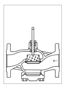
Section of pressure-balanced valve with perforated plug
