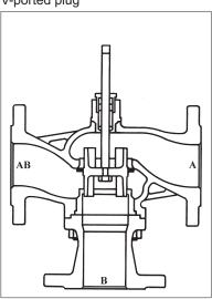
Section of valve with perforated plug
